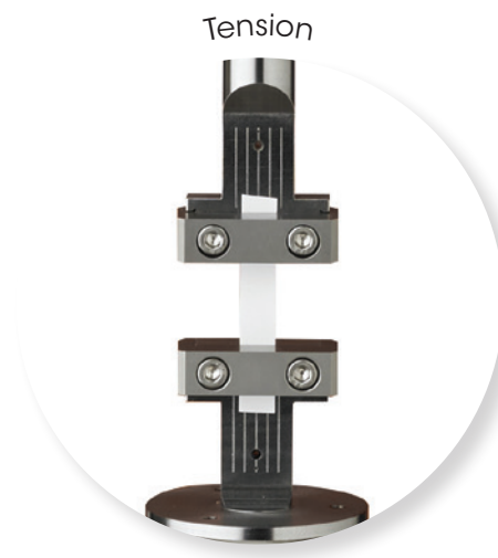
PET Film - Tension 50 μm thick
